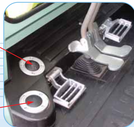
Single-action auxiliary circuit with pedal
